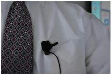
16. Turn the transmitter switch to the ON position. The red battery (BAT) light should become green after a couple of seconds.
