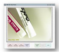
5. **To darken or lighten the document or object** the **Iris/Color** buttons open or close the iris of the document cam and allow you to darken or lighten the object(s) being displayed. This is useful to diminish glare from sun shine through the classroom blinds or from the fluorescent lights when it is necessary to keep them on for note taking.
